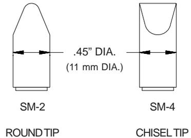
The Superline is a pocket size marker. This marker is constructed from precision machined, anodized aluminum components and can be completely disassembled for cleaning and repair. A pocket clip is snapped onto the slip cap so it's with you when you need it. To insure the valve won't leak during operation we use a viton o-ring. Use Universal Type FD ink for marking on both porous and non-porous materials.
