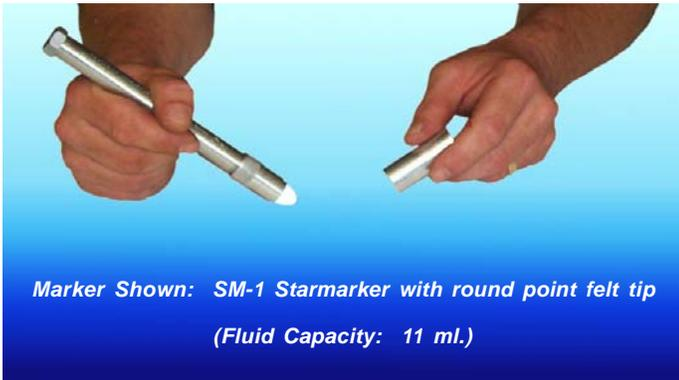
The StarMarker is the finest quality industrial fountain marker on the market. This marker is constructed from precision machined aluminum components for durability and can be completely disassembled for cleaning and repair. Pressing down on the felt tip opens the valve and feeds ink to the tip. A viton o-ring ensures leak proof valve operation. Use fast drying Universal Type FD ink for marking on both porous and non-porous materials.
