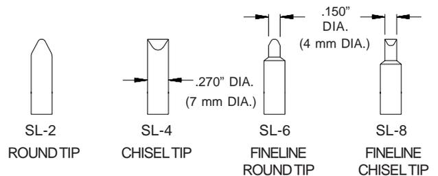
The Superline marker uses interchangeable felt tips which thread into a receiver in the valve assembly. The wide variety of available replacement tips make this marker more versatile. Replacement felt tips are packaged in quantities of one dozen per package.
